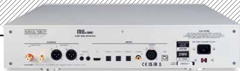
ABOVE: The M8x DAC offers USB-B (768kHz/24-bit and DSD512), AES/EBU, coaxial and three optical inputs (192kHz/24-bit and DSD64) alongside RCA and balanced XLR outputs. The HDMI/I 2 S socket carries a 16.9344MHz clock output to synchronise with future products while 12V trigger ports service full system integration
