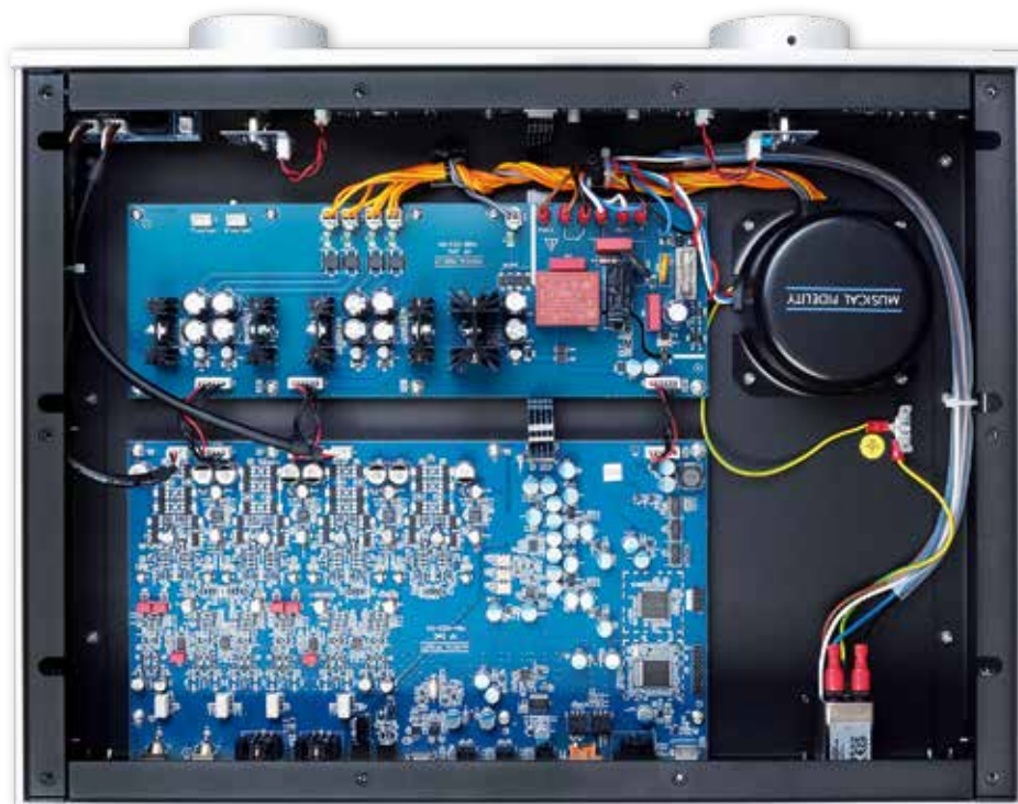
RIGHT: Linear PSU [top and right] feeds the XMOS USB/Altera DSP/ES9038Q2M DAC-based digital stages [far right], and fully balanced, discrete component headphone amp [mid left] and main analogue output stages [lower left]
