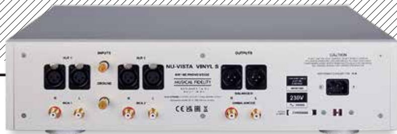
ABOVE: The Nu-Vista Vinyl S hosts two sets of single-ended (RCA) and balanced (XLR) inputs and one set of RCA/XLR outputs (the XLR inputs are suitable for MCs only)
