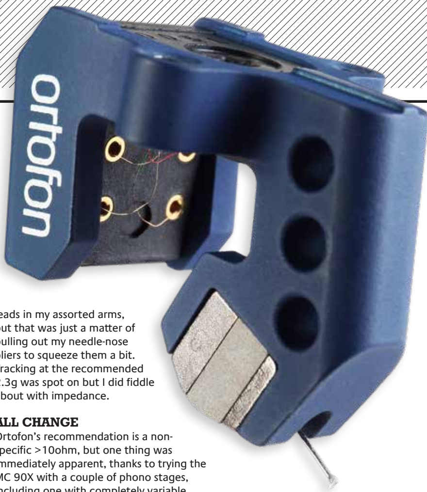
LEFT: Threaded lugs and three-point headshell mounting are revealed alongside the exposed, gold-plated 6N copper coil and lead out wires. The Ortofon Replicant 100 stylus is glued onto the boron cantilever (see also inset shot, below)
