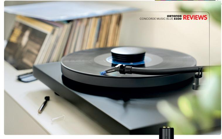
cantilever). Whichever version you buy, you can swap it to any other just by replacing the stylus. Recommended tracking force is 1.8g and dynamic lateral compliance is 15  $\mu$ m/mN, a medium-ish figure that's ideal for most tonearms. Total weight is 18g, so it should balance in most arms easily. Recommended loading is between 150 and 300 picofarads, at 47kohms. Ortofon claims a frequency range of 20Hz to 20kHz (at +2dB and -1dB respectively).
