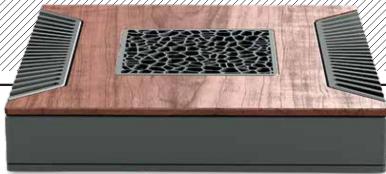
ABOVE: The Nucleus Titan's new 6cm-high machined aluminium casework, offered in wood [pictured], metal or stone 'elemental' finishes, incorporates side-mounted heatsinks and a perforated inlay as part of its passive thermal management
