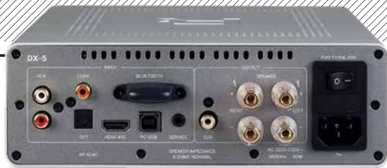
ABOVE: An analogue line in, and sub line out, are joined by Bluetooth (aptX HD/AAC), optical/coaxial (192kHz/24-bit), USB-B (384kHz/32-bit, DSD256) and HDMI ARC digital inputs. A pair of speaker outputs are offered on 4mm cable binding posts
