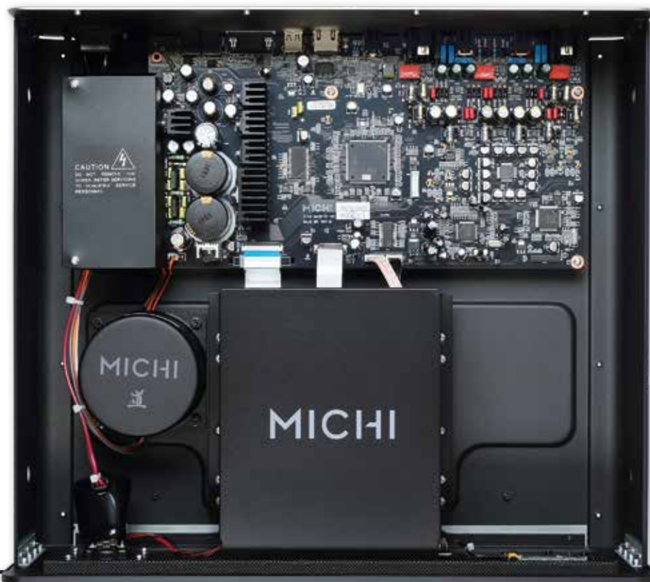
RIGHT: Linear PSU [left] feeds regulated supplies for the custom CD drive [bottom] and mainboard with its STMicroelectronics controller [top centre], ES9028PRO DAC and balanced analogue output [top right]
