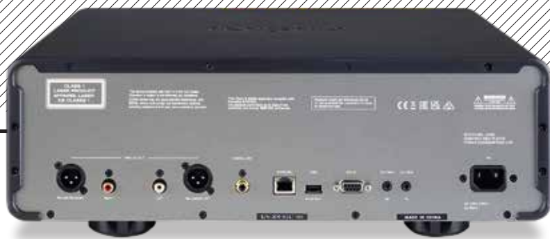
ABOVE: Fixed line outputs are offered on RCAs and balanced XLRs alongside a coaxial digital output, Ethernet port (firmware updates and connection to the CD database), USB-A port (firmware updates) and RS232 / 12V trigger ports (system control)
