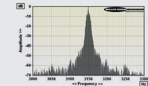
ABOVE: Wow and flutter re. 3150Hz tone at 5cm/sec (plotted ±150Hz, 5Hz per minor division). Absolute speed is very accurate indeed
