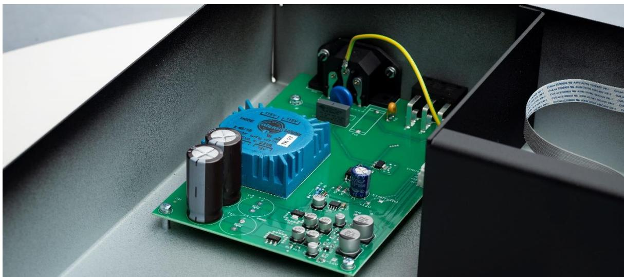
The special audio transformer with low core saturation utilised within the M3x Vinyl decreases the level of electromagnetic radiation, which is essential for proper operation. Internally, the M3x Vinyl affords space between the transformer and the amplification section inside the chassis, while also installing electromagnetic shielding for extra protection. The result is an incredibly high signal-to-noise ratio, for absolute clarity in sound.
