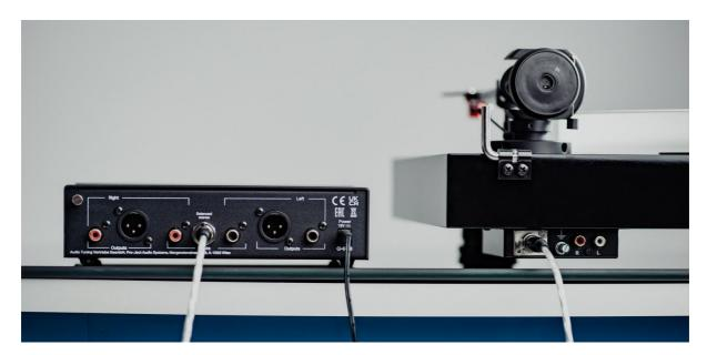
Supplied with an Ortofon Quintet Red moving coil cartridge pre-installed, the X2 B is capable of benefiting from Pro-Ject's *True Balanced Connections* concept. By connecting to a balanced-capable phono stage (Pro-Ject Phono Box S3 B pictured) using the mini-XLR output on the back of the turntable, you can benefit from increased dynamics, less noise and improved signal-to-noise ratios. Going true balanced is like hearing parts of your music that were not there before.
