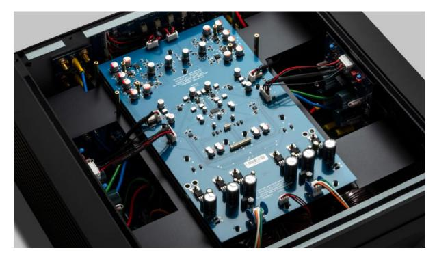
The benefit of this new top-layer PCB design is that there is more space in the chassis for connections, so the Nu-Vista 600.2 boasts six stereo inputs, including two balanced XLR inputs. There are also three
