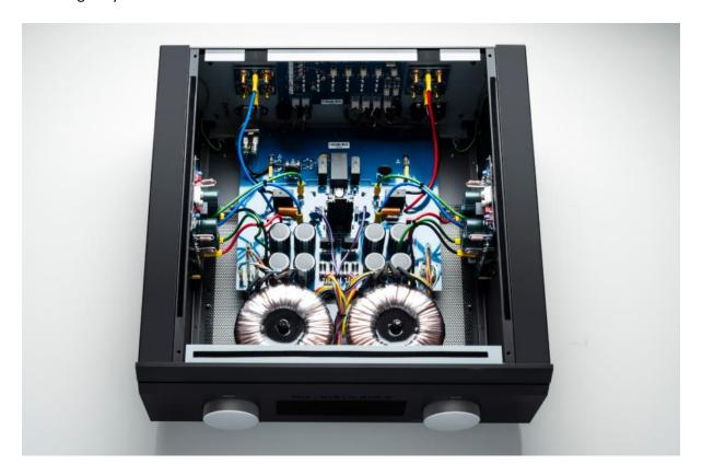
In typical *Nu-Vista by Musical Fidelity* style, the overall construction of the Nu-Vista 600.2 is uncompromisingly solid. The front and side panels are milled from extruded aluminium profiles, contributing to a chassis that effectively acts as a Faraday cage, protecting the internal circuitry from external electromagnetic fields. Because of the overall weight, the chassis is also resistant to other mechanical vibrations and airborne interference.
