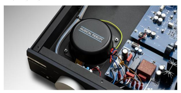
The M8x Vinyl's discrete power stage, featuring an encapsulated super silent power transformer, is designed with care to ensure it generates as little noise as possible. Further, industrial grade power sockets with EMI filters and DC blockers stop interferences and eliminate transformer hum. The preamplifier stage is powered by two high-quality symmetrical low-noise power supplies - one for each channel – which are both passively filtered and regulated.
