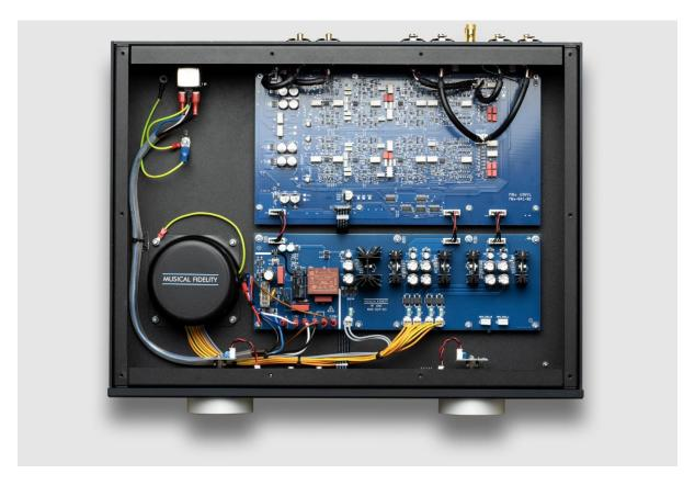
The M8x Vinyl is both fully discrete and fully balanced, which means that there are no integrated circuit chips used in the audio signal path, and for all the selected components, double the amount are used to make it fully balanced. The result is a purer signal path, which results in a natural, dynamic musical performance free from noise.
