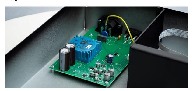
The special audio transformer with low core saturation utilised within the M3x Vinyl decreases the level of electromagnetic radiation, which is essential for proper operation. Internally, the M3x Vinyl affords space between the transformer and the amplification section inside the chassis, while also installing electromagnetic shielding for extra protection. The result is an incredibly high signal-to-noise ratio, for absolute clarity in sound.
