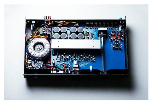
The 1980s blueprint directly inspires the new A1's transformer design; however, Musical Fidelity updates the system with more efficient dual-mono split-rail windings and superior components, improving stability and heat management. Fully independent supplies for the left and right channels now power the amplifier, bringing better power handling and stereo imaging. Each power amplifier now has double the supply capacity, reducing ripple and noise artefacts.
