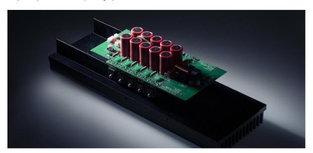
Elsewhere in the circuitry, chokes are added for further-improved supply ripple. Pulse current spike reduction bias is set for over 5W of initial Class A operation that slides into Class B operation at the point where the lower discontinuity is easier dealt with than "standard" crossover distortion. But the extra secret behind the overall performance is found in the large external power supply unit that accompanies the Nu-Vista PAS.
