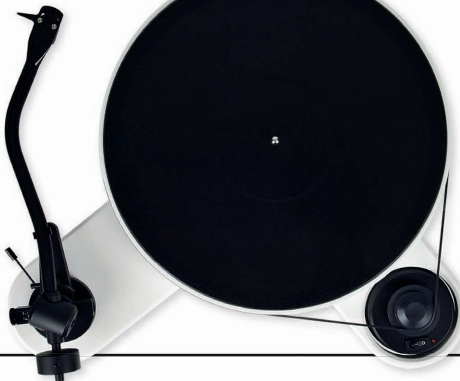
**RIGHT:** The motor sits in a dedicated hole in the plinth, offering manual speed change for 33 and 45rpm via a stepped pulley. Vinyl topped MDF platter is dynamically balanced at the factory
