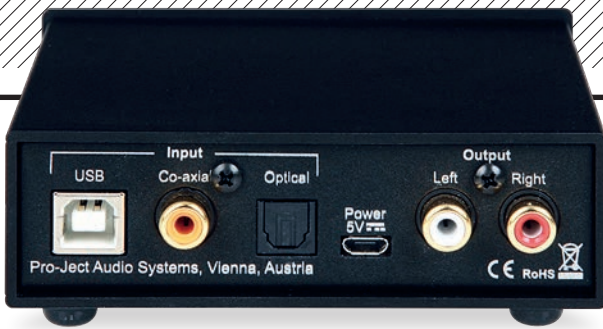
LEFT: USB, coax/optical digital ins join variable analogue outs on RCAs. Note micro-USB port (5V PSU)
