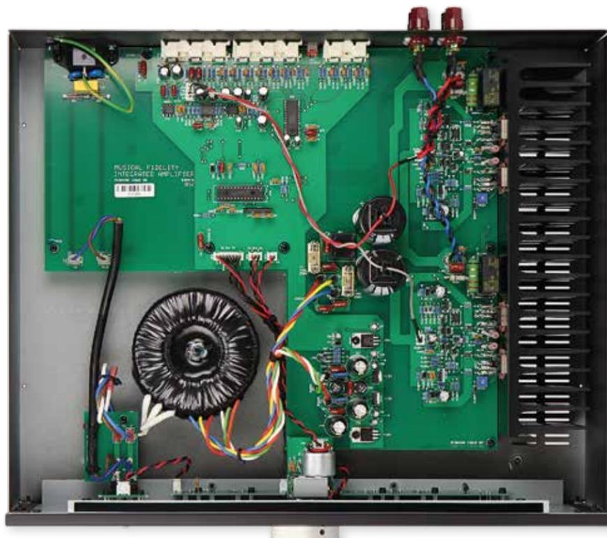
**RIGHT:** The M2si includes a toroidal transformer and linear PSU [lower left and centre] feeding a discrete output stage with one pair of devices per channel [on heatsink, far right]. Note motorised volume control [bottom]
