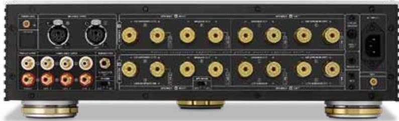
**ABOVE:** The one balanced XLR/three RCA line inputs are joined by an MM/MC phono input, subwoofer output and no fewer than 16x 4mm speaker cable posts. There are both A and B speaker banks with two amplifiers per 'channel' (one with optional high-pass filter) for either bi-amping or bridging into two, single channel amps
