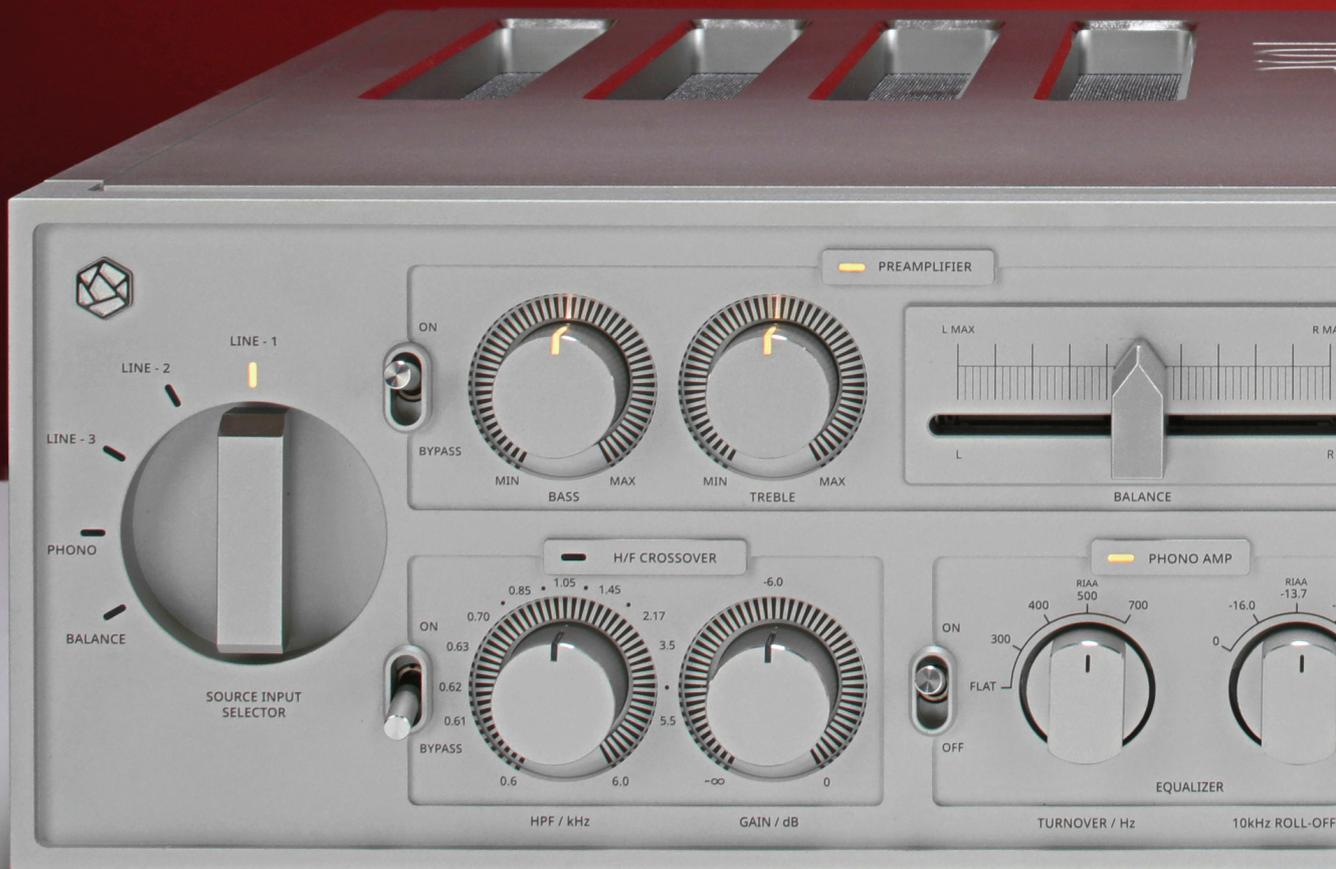
These unusual features of the RA180 explain all the front panel controls, if not the adornments. There are bass and treble tone controls that can be switched out, a 'high-pass' tuning section that can be switched out, a complex Phono preamp section, a slide control for channel balanced and – yes – that funky volume control with its gears, back illumination and physical pointer to show volume level. Whoa! Behind lies a motorised potentiometer that can be remote controlled.
