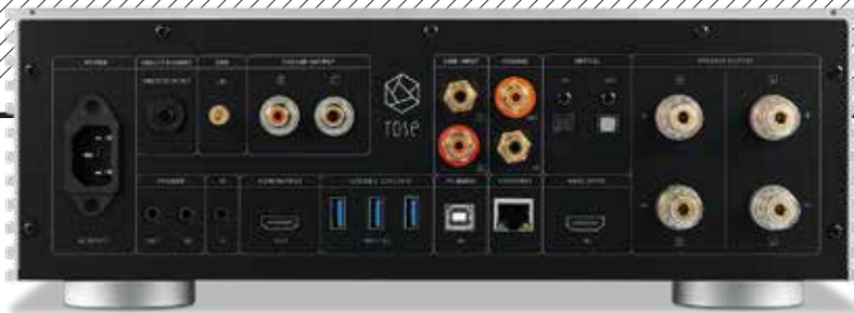
ABOVE: Line in/pre out (RCAs) are joined by optical and coaxial digital in/outs, HDMI in/outs (with eARC), an Ethernet port, three USB-A ports for external media and one USB-B for computer connection. Loudspeaker cable is connected via 4mm terminals
