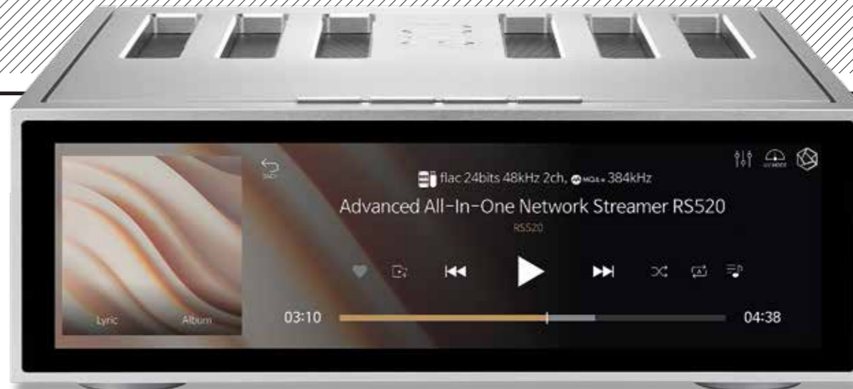
LEFT: The RS520's 12.6in-wide touchscreen TFT display provides fingertip control over everything from input selection to menu setup, supplementing the Rose app and IR handset [p53]
