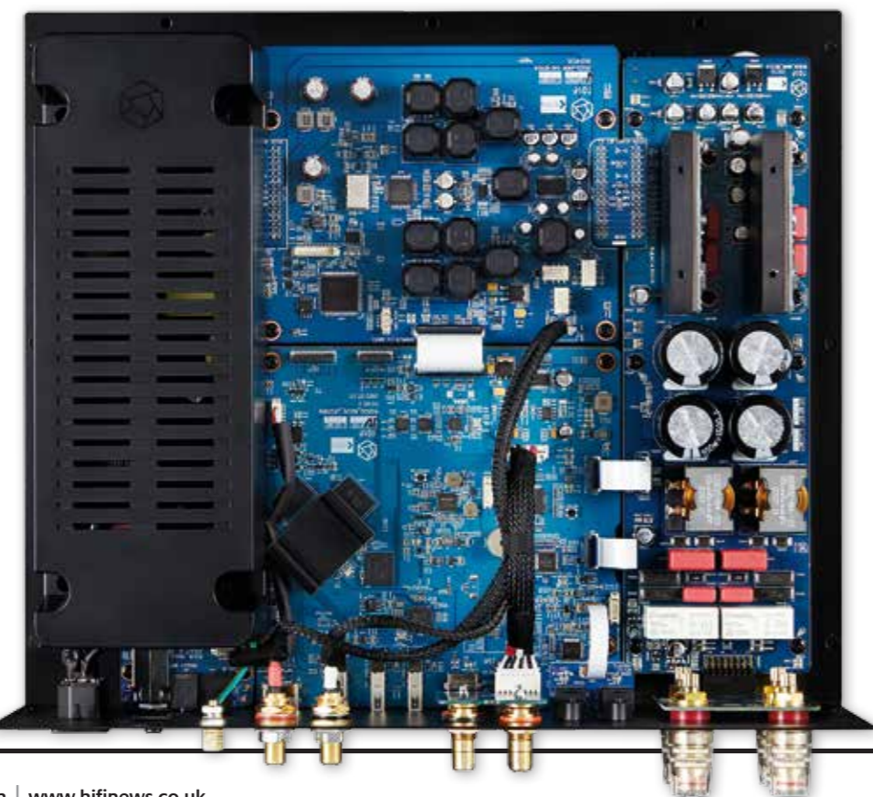
RIGHT: Screened switchmode PSU [left] feeds Cortex hexa-core CPU [lower left], ES9038PRO DAC and preamp stage [top centre] and GAN-transistor Class D power amp/filter block [right]
