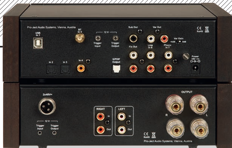
ABOVE: Line and phono analogue ins are offered alongside coax, USB, wireless Bluetooth and two Toslink optical digital ins, with fixed/variable analogue, sub plus optical outs [Pre Box, top]. The Amp Box [below] has line in/loop outs on RCAs and 4mm speaker terminals. Note the three-pin DIN 48V PSU connection
