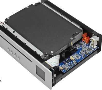
Most of the electronics live under the bought-in mechanism, which sends recovered digital audio data to the small board on the right. This contains two Burr-Brown chips.
