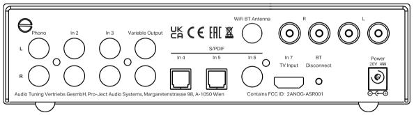
1. Make all connections except the connection to the headphone whilst the unit is disconnected from the mains.
