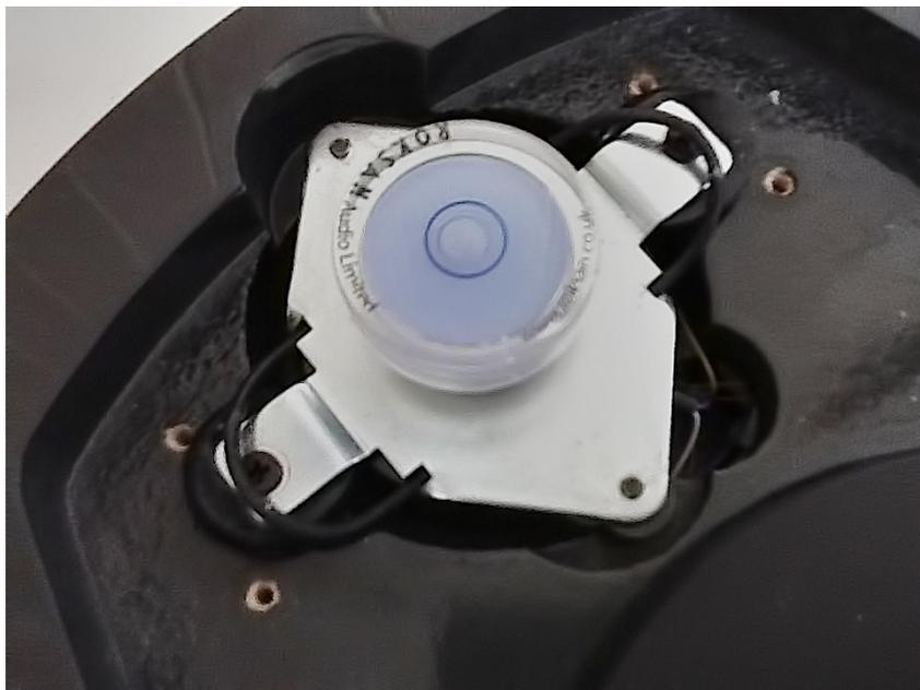
Using a spirit level to balance the motor mount (note the new grommets and black screws)
